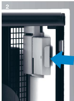
Insert the Air Intelligence Module into the module holder.
