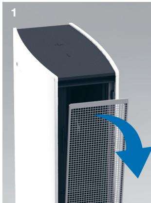
Turn the unit off and open the intake door by pulling at the top edge. The intake door is on the right hand side when facing the front of the unit.
